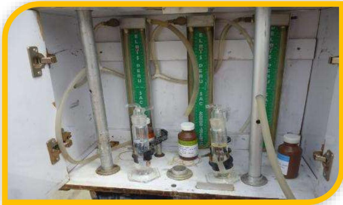
Imagen 10.- Solución captadora SO<sub>2</sub>
